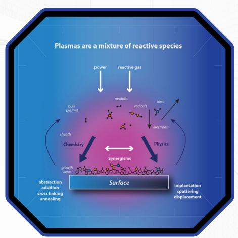
A plasma contains positive ions, electrons, neutral gas atoms or molecules, UV light and also excited gas atoms and molecules, which can carry a large amount of internal energy (plasmas glow because light is emitted as these excited neutral particles relax to a lower energy state). All of these components can interact with the surface during plasma treatment. By choosing the gas mixture, power, pressure etc. we can quite precisely tune, or specify, the effects of the plasma treatment.
